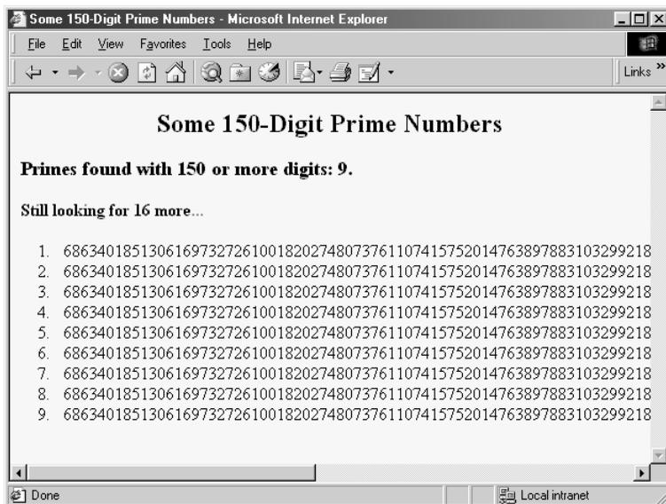
**Figure 7-2** Intermediate result of a request to the PrimeNumbers servlet. This result can be obtained when the browser reloads automatically or when a different client independently enters the same parameters as those from an ongoing or recent request. Either way, the browser will automatically reload the page to get updated results.
