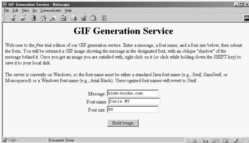
**Figure 7-5** Front end to ShadowedText servlet.
